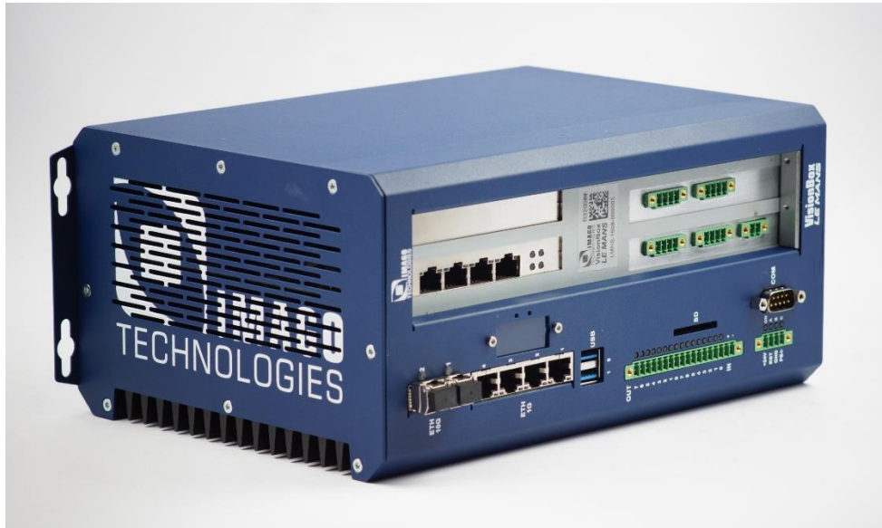
Fig. 6: The VisionBox LE MANS with 10 GBit/s Ethernet, PoE, ToE, LED Controller
