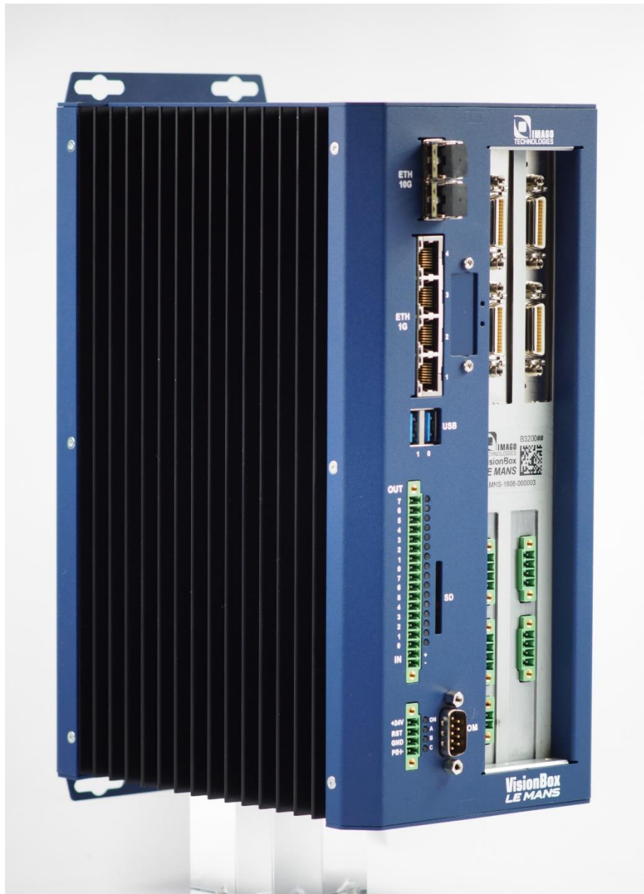
Fig. 8: For line scan camera applications: LE MANS incl. Camera Link Grabber
